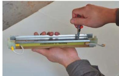
2. Remove the pressing stick from the complete sealing bar by cross screwdriver, then remove the stainless steel base.
