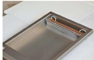
12. Connect the cable of the complete sealing bar to the pin, then put the sealing bar back in the vacuum chamber to complete the installation.
