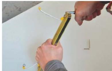
7. Fasten the heating wire, then cut the excess heating wire.
