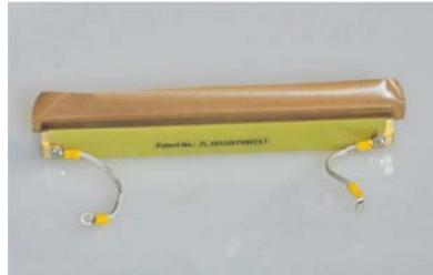
8. Take the new sealing tape at a proper length and stick it on the heating wire.
