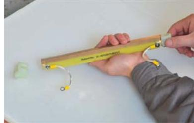
10. Put plastic clamps on the sides of the sealing bar.
