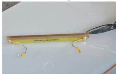
9. Cut the remaining sealing tape on the ends to allow them to fold over.
